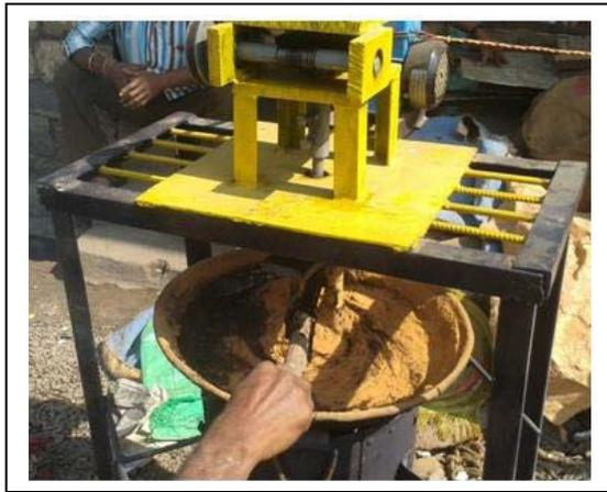
Figure 4. Early trials of planetary stirrer.
